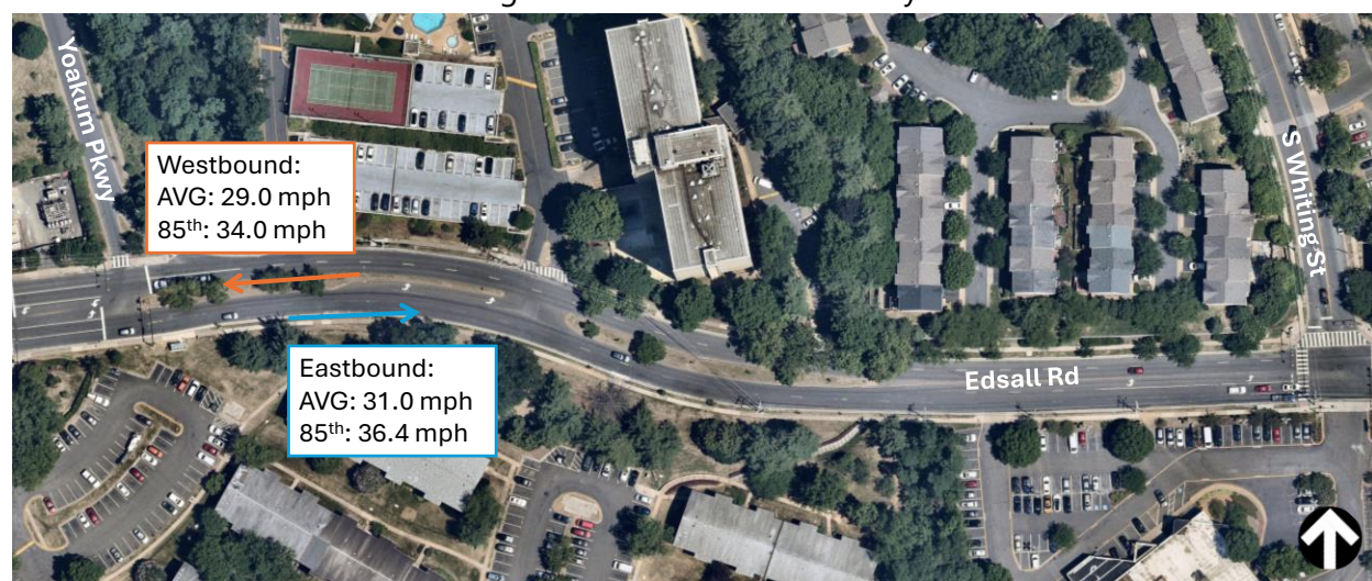
Figure 15. Average and 85 th Percentile Speeds between S Whiting Street and Yoakum Parkway
