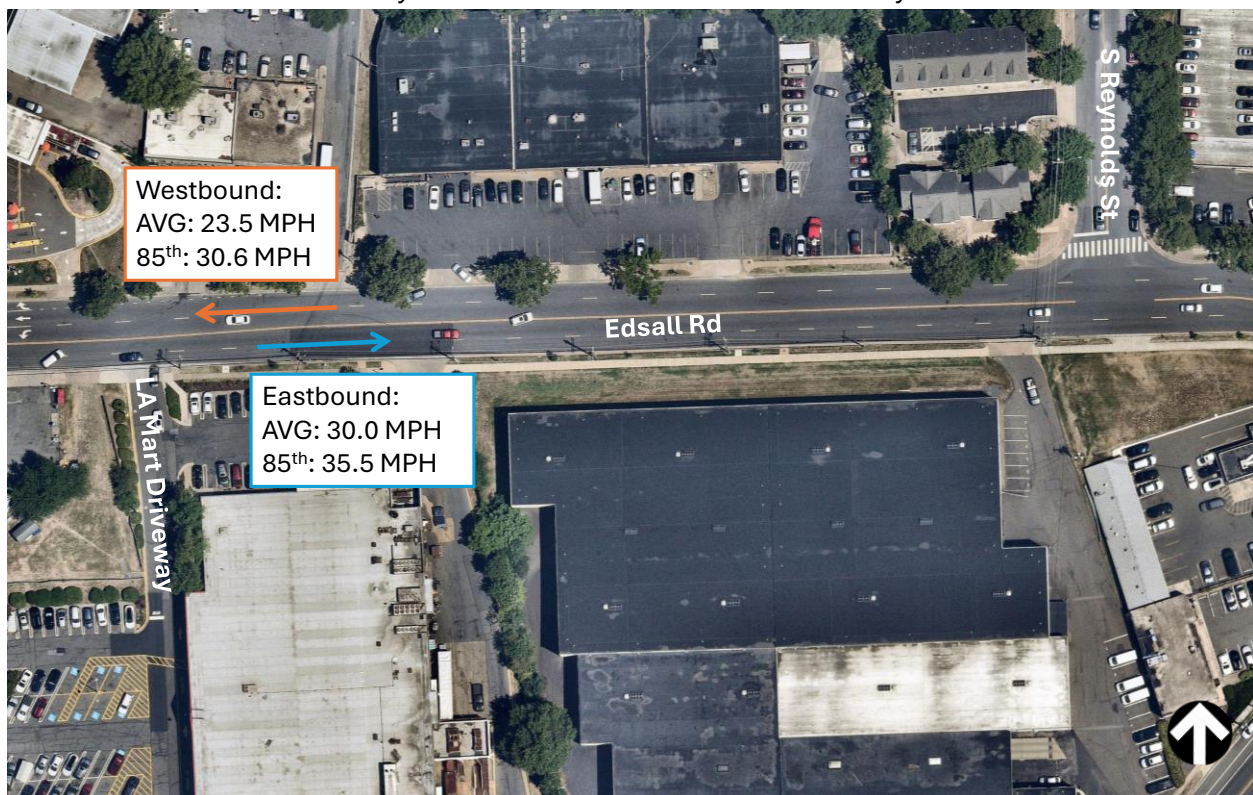
Figure 14. Average and 85 th Percentile Speeds between S Reynolds Street and LA Mart Driveway
